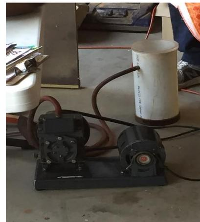
Shone on right is a vacum pump and vacum chamber fabricated from a section of PVC pipe and fitted with an hose connection and a Lucite cover gasket
