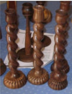
**Rick Haseman:** A series of Legacy turned candlesticks with a barley twist body. The hole for the candle is started at  $\frac{3}{4}$ " and after the piece is finished, the hole is tapered using a modified  $\frac{7}{8}$ " spade bit. He side grinds the spade bit from a bit less than  $\frac{3}{4}$ " to a full  $\frac{7}{8}$ ". This is then used to taper the candle hole.
